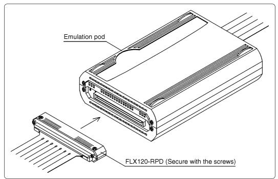
Figure 3.8 Connecting the emulation pod and FLX120-RPD
